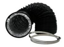
Eliminate Fan and Airflow noises in your ventilation system with our premium quality sound trap ducting. Combi Flexible Duct is a combination of an aluminium/ polyester laminated innerduct with a high tensile steel wire helix, covered with a mechanical resistant PVC layer.
